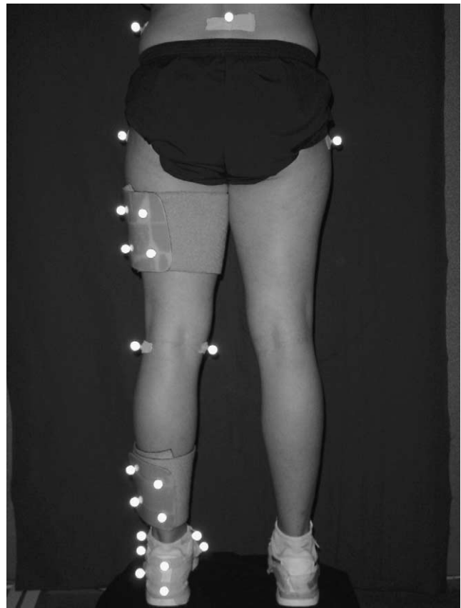
Fig. 1. Retro-reflective marker placement on the tested lower extremity.
